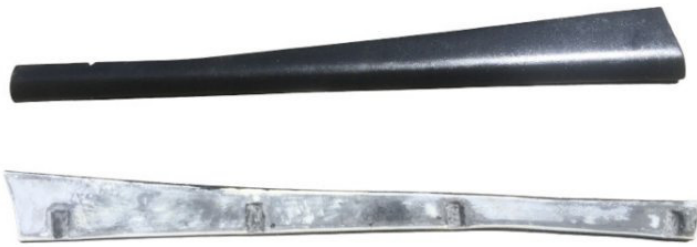
The bottom panel upped the rigidity enormously. I'll be using M6 studs in the body, sliding the four holes over them and attaching the boards with wide washers and stainless nuts. Rivnuts at each end will provide attachment to the guards.
