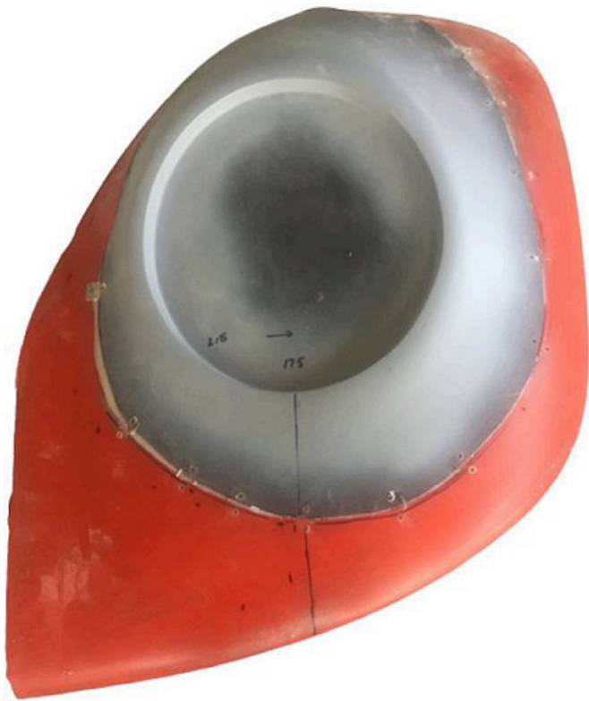
This is how I converted upright-headlight mudguards to sloping ones.
