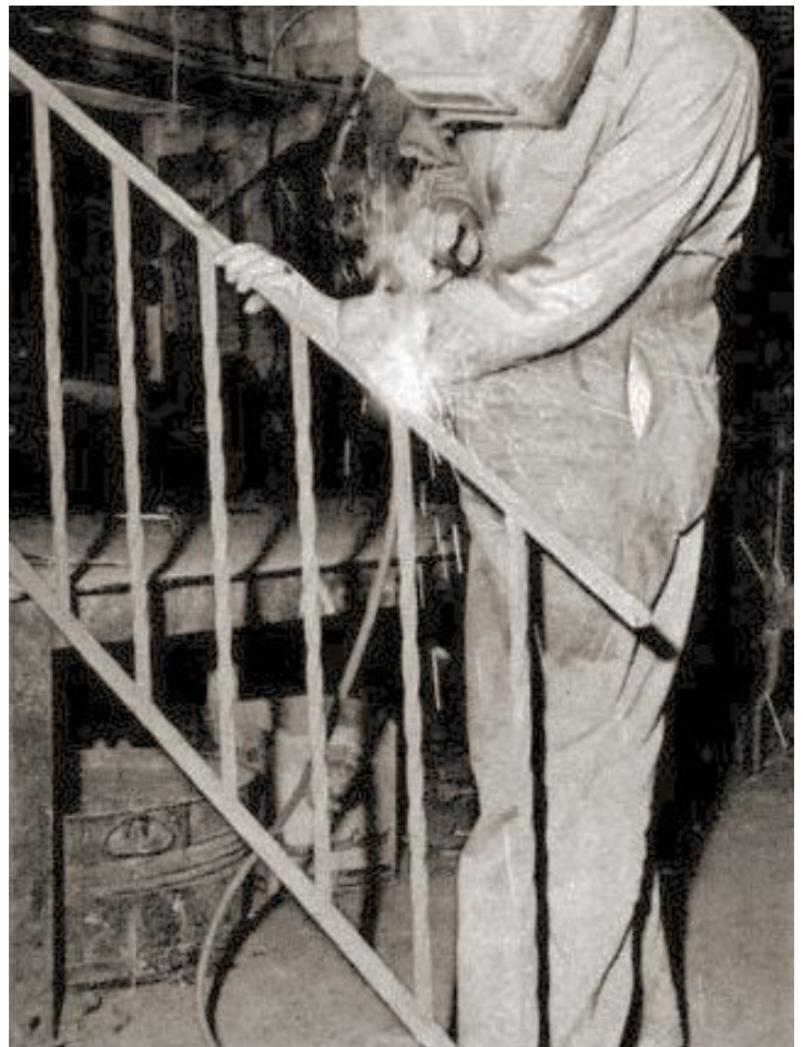
HOT-ROLLED MILD STEEL is too low in carbon content to harden when heated. Tough, it can be twisted or bent; welds easily. Use it for assemblies like this decorative stair rail.
