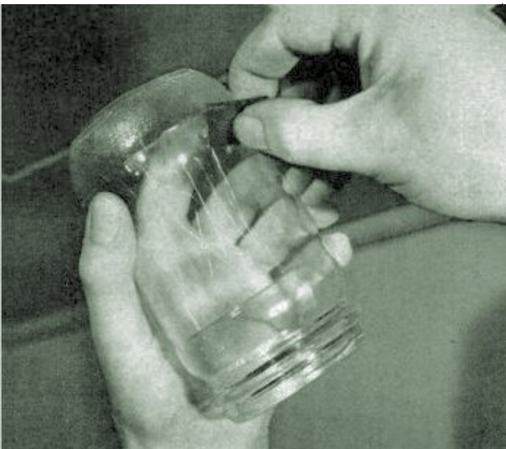
SCRATCH TEST. Draw a corner of the hardened sample across a piece of glass. Fully hardened, high-carbon steel will leave scratches in the surface. This kind must be worked while annealed, then hardened and, finally, re-heated at about 400° to relieve internal strains.
