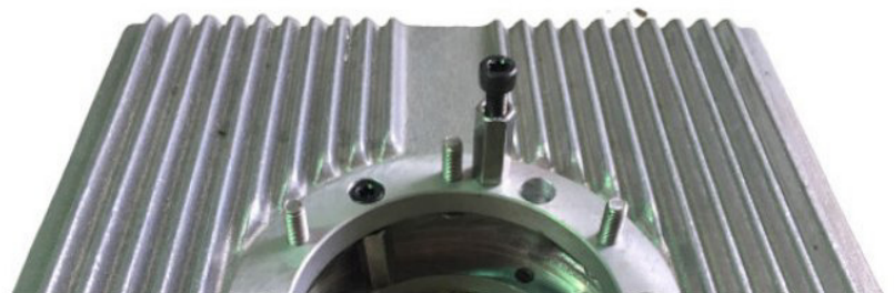
The left hole has the coupling nut and cap screw in place. The holes in the bottom of the sump needed drilling out to allow the screw heads to pass through. I will also be using these Torx socket-head cap screws for securing the tinware.
