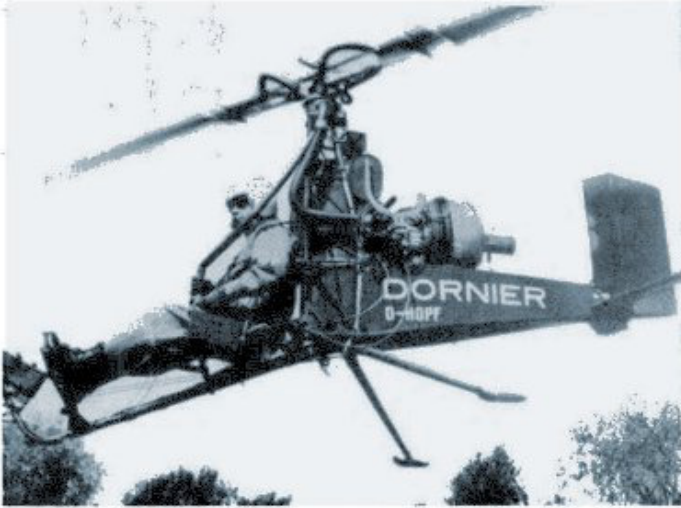
Turbine, behind pilot, burns gas, diesel oil, other fuels.
