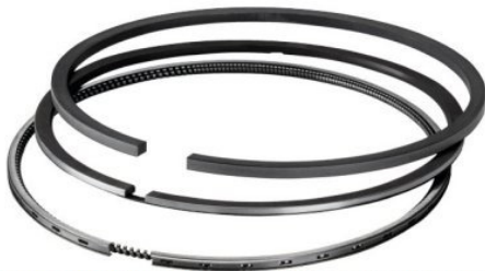
The second ring has a very thin, additional ring which sits inside the main ring. Each of its gaps is set at 180° from its counterpart, ensuring minimal compression leakage.
