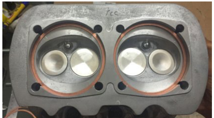
copper rings in place
