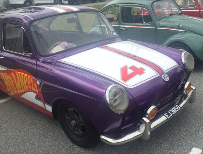
Another owner with the bright idea of retrofitting sloping headlights to an early Type 3, this time with 911 glass.
