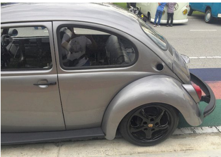
Beautiful job on these additional air inlets, but I fear that air would be sucked out, rather than in.
