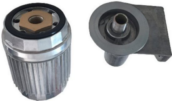
The newly machined nipple was Loctited into place and the filter now spins onto it and seals like a charm. Nipple nipple nipple.
