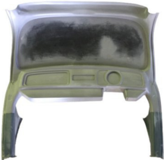
Dash with panel for AC vent outlets and grafted-on pillars
