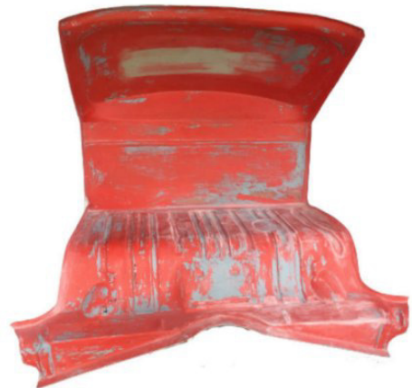
Temporary product of the cargo deck. The groove for the wiring harness is visible on the right. I'm reproducing another one on the left. I corrected the bottom-most strips by flattening them out.
