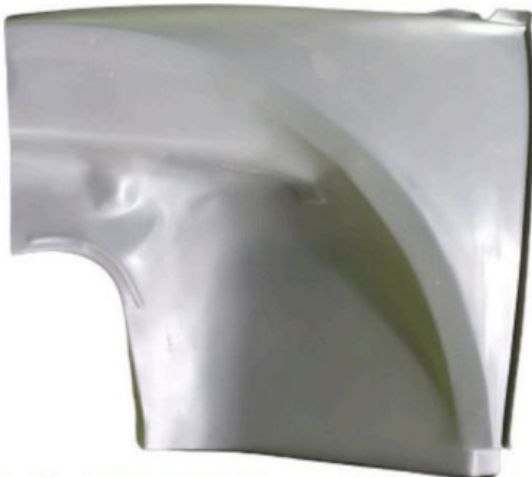
The front part of the inner side panel is accident-damaged, so I could only make a mould of this much of it.
