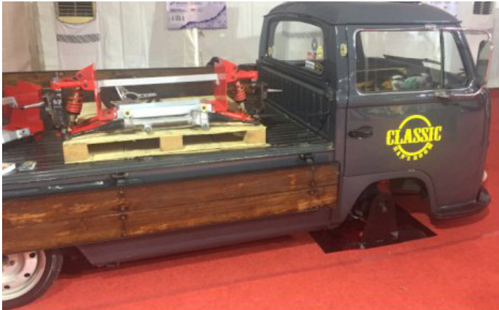
A bolt-on unequal-length A-arm front suspension for T2s, complete with rack and pinion, progressive coil-overs and discs. Wow.
