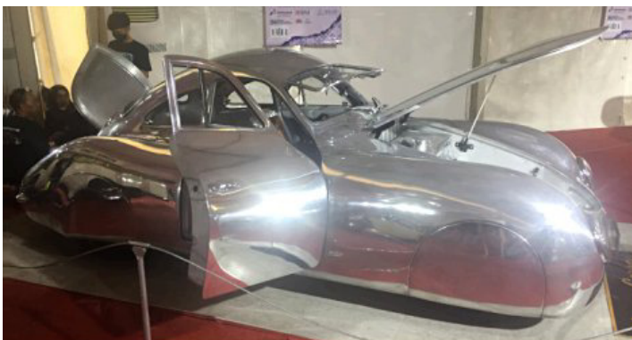
A replica of the Ur-Porsche, the Type 64, or Berlin-Rom-Wagen, painstakingly hand-beaten from aluminium. You don't see one of these every day.
