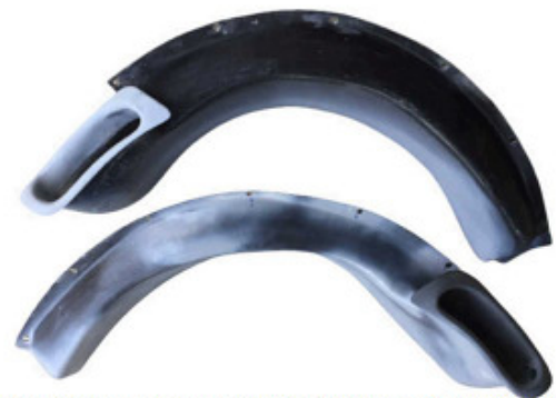
The air inlet is at the base of each mudguard, imitating a Porsche 911 shark-fin stone guard. A hole at the other end will communicate with the engine bay, supplying copious amounts of lovely cool high-pressure fresh air.
