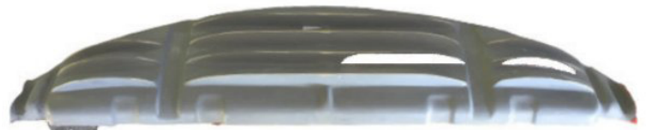
Prototype of my heavily bogged-up, improved louvre panel with 14 larger entry points. I measured the whited-out areas which represent factory holes.
