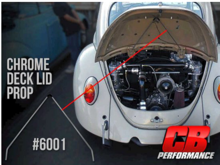
Gravity and the spring exert too much force on fibreglass pieces, so this thing will hold up my lid.
