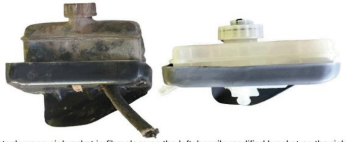
stock reservoir bracket in fibreglass on the left; heavily modified bracket on the right
