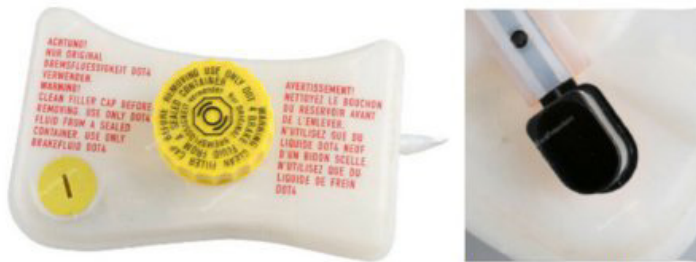
the missing electrical connector socket on the right
