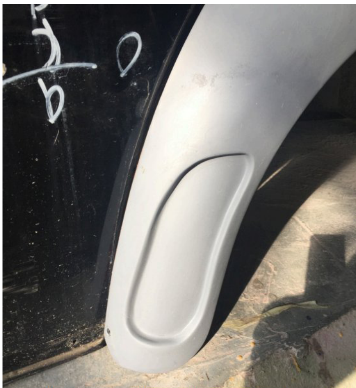
A project in progress: this is where air will enter at the base of the mudguard.
