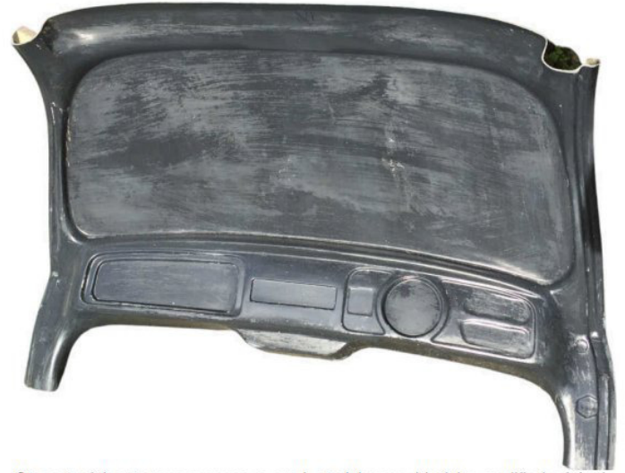
Stage 3 of the 5-stage process: a product of the mould of the modified original.
