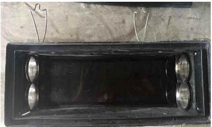
The inside of my box showing cut-off and lengthened 2-inch velocity stacks
