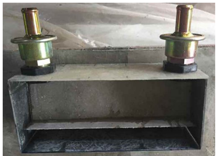
A work in progress: the "penthouse" box. There will also be fittings sending air to the valve covers and the idle-air control valve.
