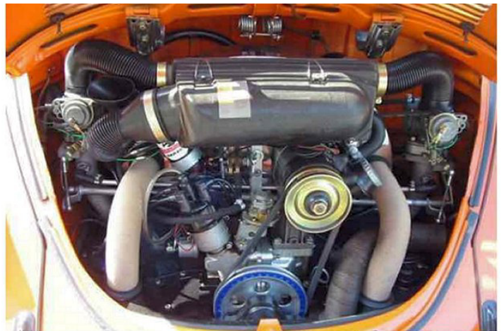
Oettinger's installation of a standard filter box combined with a redesigned filter base
