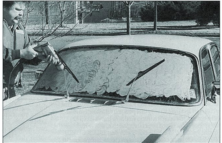
Felt polishing wheel and oxide powder slurry can buff out windshield scratches.
