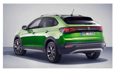
The new coupe-inspired Taigo model blends the T-Cross and Polo's sharp styling elements - including the former's upper grille design and full-width rear tail-light signature, and the Polo's side doors, windscreen, roof stamping, suspension setup and most interior parts for efficiency and cost-cutting measures. It has a unique dash and lower bumpers and a roof that begins a steep slope from the C-pillar back.
