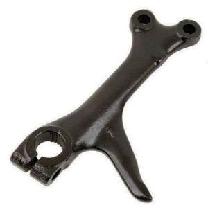
o Would someone please explain to me why the hole where the short tie rod fits on the Pitman arm is further outboard than the one where the long one goes? Is it the only way to maintain proper Ackermann geometry with an offset steering box? I have never seen or heard an explanation.
