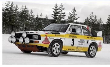
Sport quattro added a 20-valve twin cam head that kicked power up to 225 kW and 350 Nm in the 200-odd road cars that were required under Group B homologation, but tuning of this package for the rally cars delivered at least 300 kW and up to as much as 400 kW.
