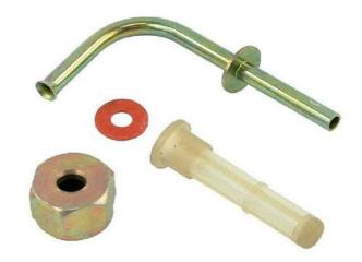
o The outlet pipe on the fuel tank. Why does it have to have an extension on it? With the extra length in place, the tank volume is effectively slightly smaller. The inevitable water which collects does not get pulled through to the carburettor or injection, for a while anyway. It sits there unsuspected and has its evil way with the steel. The ensuing rusty tank can't be fixed safely.
