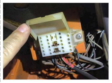
o The VW Diagnosis system. It was ahead of its time. Why was it dropped after such a short time? VW stated that it gave false readings. I would like to know what specifically failed. It did entail quite a bit of extra cost per car and a special battery with a centre tapping.
