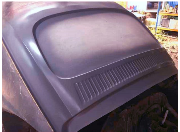
Details of the my reshaping of the opening around the rear window. I deserve a medal for blocking up those air-inlet slots.
