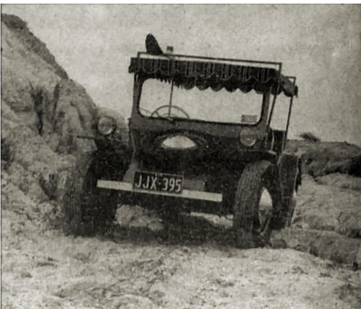
Parts are all VW. Conventional body can be just lifted off, steelfast type replaced. Go anywhere ability is almost as good as Land Rover.
