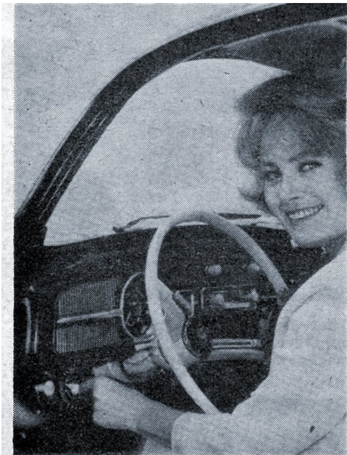
Setting the time switch (above) of the Eberspacher heater unit fitted to a Beetle (lefthand drive German model) which ensures a completely pre-heated car within any given time.
