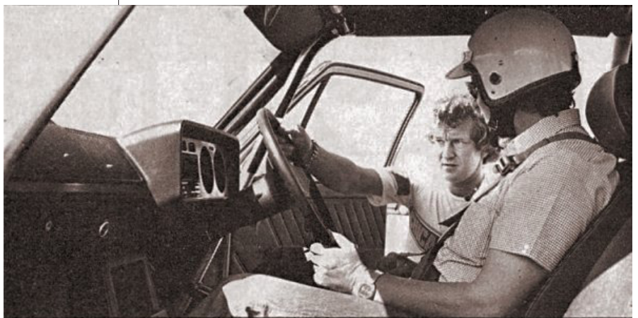
McCarthy gets cockpit drill from Chris Heyer. Interior is standard Golf aside from roll cage, six-point harness, fleecy seat cover and oil pressure gauge.
