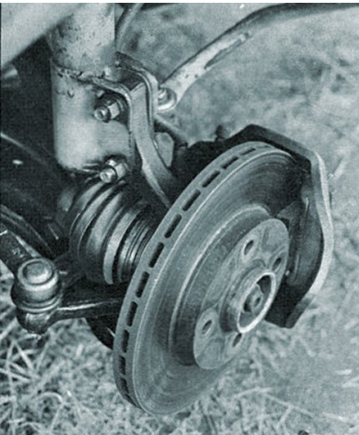
GTI has stronger driveline and ventilated front discs.
