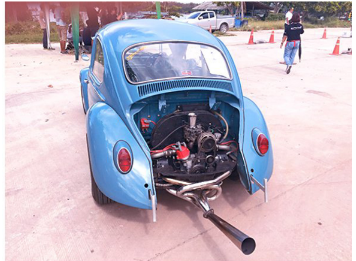
This Beetle was consistently the quickest all day, even though it's limited by a 34PICT. There is a special class where you can do any engine modifications except for the stock carburettor.
