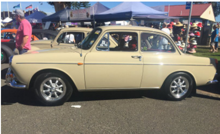
THAT projecting boot is a phony, made up of plastic and foam rubber — back is like a Mini's, but with a bit more slope. Peeling camouflage in the big photo reveals true shape of rear side windows. Engine stays at back; wheels are 12 in.
