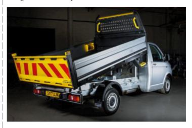
Created and developed in partnership with Volkswagen Commercial Vehicles (UK) by Ingimex Ltd – the UK's largest manufacturer of light commercial vehicle bodies – the tipper body conversion is available for both T30 (3000kg GVW) and T32 (3200kg GVW) versions of the Volkswagen Transporter, offering payloads of around 800 kg and 1000 kg, respectively.
