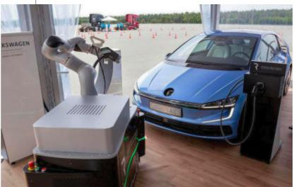
Most interestingly, the Gen.E can be recharged via a specially designed robot, which VW is developing to work in underground and multi-storey car parks to help automatically connect electric vehicles up for recharging.
