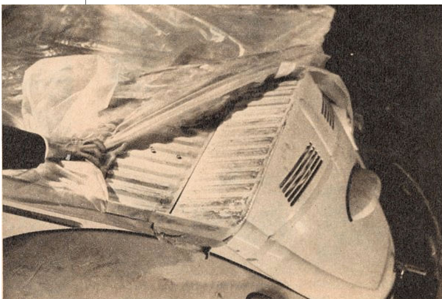
CARGO well has a lip around it and a metal cover, so it can serve as a tray for additional loads. Air intakes are transferred to engine-bay lid.
