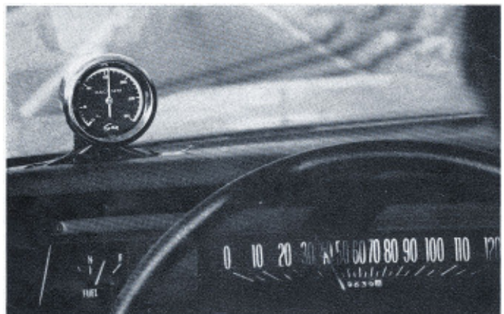
Mounting gauge atop dash, in line of sight, makes fuel-minding more effective, but takes extra hardware. Most gauges have in- or under-dash mounts.
