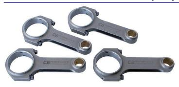
angle is increased. 78 mm is the maximum that the stock rod can withstand; beyond that the bolts will fail. Longer crankshaft strokes require a longer connecting rod, and/or a stronger or a better-designed rod connection system. This is exactly what 4340 Chrome-moly rods accomplish.
