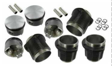
**88 mm**: The next bore size up from stock is the machine-in 88 mm set. These work VERY well, but you are looking at a lot of machining (this costs approx. \$200) for a very small displacement increase! If you're going to go to that work or expense, you should opt for the larger piston set. However, 88s are very good for Buses and Type 3 engines, since these engines run hotter than Beetles, Ghias, or buggies/rails.
