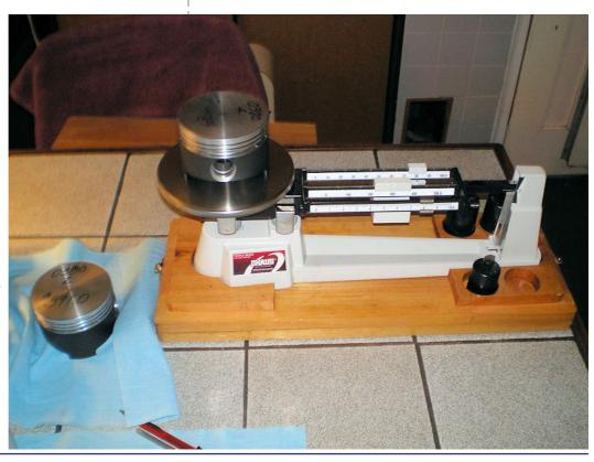
In the final stages, each time you weigh the piston you must make sure it is clean. The residue of metal you're removed will try to cling to the piston. It will get into the ring grooves and wrist-pin trunnions. And when it does, its weight will still be there.
