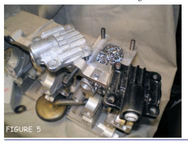
identical, purchased for about \$5 each. The one on the left is as-received, the one on the right has been bead-blasted then treated with a thermal dispersant. (Tech Line's 'TLTD').
