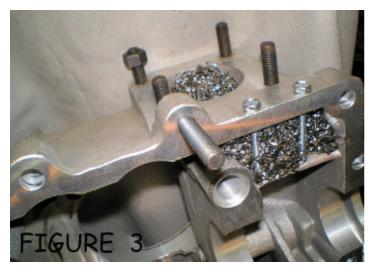
You want the mesh to pretty much fill the D-shaped hole for the dynamo tower but not to bulge above it. That will allow you to use an inexpensive oil pump cover as your outlet. Nor do you want it hanging out the bottom. This is the cam-gear gallery and the last thing you need is to have your mesh get sucked into the gear train.
