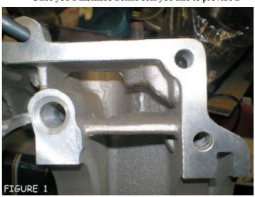
new ventilation inlet to the crankcase. Most guys plumbed a filtered line to their valve covers.
