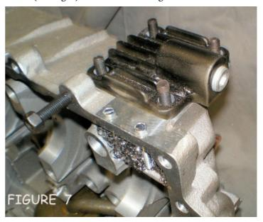
plate. On my engines I run the outlet down to the carb-heat box, where the carb provides the required negative pressure.
