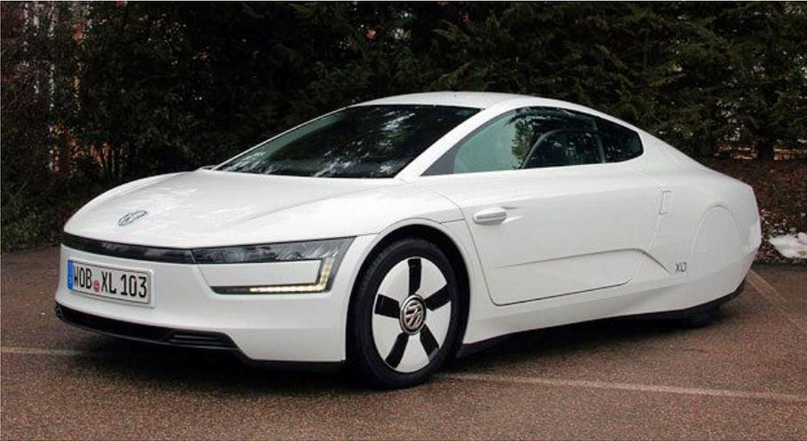
Hackenberg rejected the tandem seat as impractical, but Piëch suggested a staggered arrangement to limit the inevitable width increase. At 389 cm long and just 138 cm tall, the resulting XL1 is one of the slipperiest cars in the world, with a drag coefficient of 0.189. It is also the lightest hybrid, weighing a total of 795 kg - the resin-transfer moulded carbon-fibre body weighs just 230 kg and the entire drive system 225 kg.
