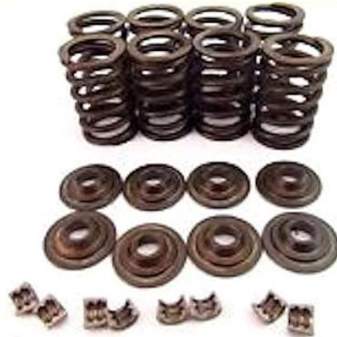
The strength of the stock VW valve spring is determined by measuring the amount of force needed to compress the spring to a height of 31.0 mm. A number of factors can affect the strength of a coil spring, and like all other VW specs, the tolerance is quite large, ranging from 53 to 62 kg force (520 to 610 Newtons, to be precise).
