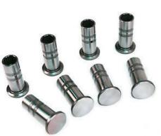
with steel. VW cams and lifters were cast iron and no one had come up with an accurate hardening process that was economical enough to be used for mass produced cast iron parts. Except an outfit called Krupp.
