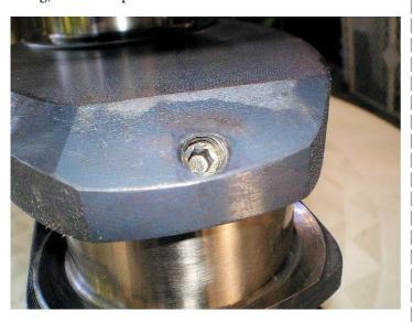
Some of the oil passages on his Chinese stroker are drillings sealed with 4 mm socket-head set-screws. They need to be pulled and the oil passages cleaned then re-installed with Loc-tite and straked. Which he hadn't done. But even as I explained the what and why I had a hunch he wouldn't bother. After all, he's built a lot of engines. And never had any trouble.
