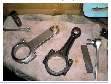
weighs within a tenth of a gram of the other. Of the two heavy rods, one is a tad less than two grams out, the other just over four. Four grams is a lot of grinding, followed by smoothing things up with the belt polisher.
