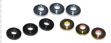
If you make up the washer so the pilot – the stepped portion -- is concentric to the bolt hole, your cam will be indexed straight up, without advance or retard. You may then install the cam and clock it. If clocking the cam sez you need to move it two degrees, you go over to the lathe and make up three new buttons with the hole offset by forty thou. That may sound like a major chore but trust me here, making eccentric buttons is a trivial task, assuming you have access to a lathe
