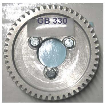
If you prefer to roll your own by modifying a stock gear (which is what I do) you'll probably find the easiest way is to use a rotary table and a milling machine, but other methods will work. I saw a guy in Baja doing a nice job on a cam gear using a router with the cam gear mounted in a wooden fixture. You wouldn't think it would work but it did a pretty good job. I guess when you don't have a shop full of tools you have to be a little smarter than the average bear.
