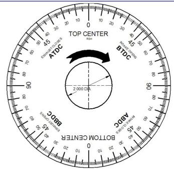
the crankshaft one complete turn from the peak should put you in the middle of the heel for that lobe. Zero your clock at that point. (Simply loosen the lock and rotate the dial until the zero-mark is aligned with the needle then re-tighten the lock. If your indicator is properly mounted it will remain steady as a rock while being zero'd. If not, it needs a better mount.)
