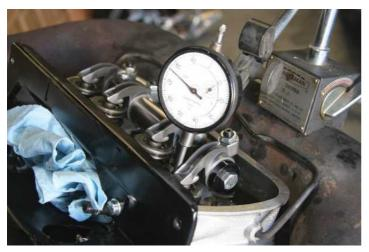
Slowly rotate the crankshaft through several revolutions while watching the dial indicator. You will see a prolonged period where the indicator makes no movement then rises, rather rapidly, to some peak value before dropping back. The prolonged period of no movement is when the tappet is riding on the heel of the cam. We need to find the middle of the heel. To do so, note when the peak reading occurs and mark that point on your degree wheel. Rotating
