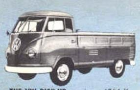
THE VW PICK-UP carries a 1764 lb. payload on a 45 sq. ft. load area — plus a weathertight lock-up compartment that provides 23 cu. ft. additional space. Sides and back can be lowered for easy loading from all sides.
