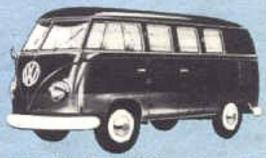
THE VW KOMBI-VAN carries 1786 lbs., has windows each side and double-doors for easy loading.
