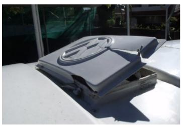
Fortunately it's only held on to the roof by two small hinges and small stainless nuts and bolts, which were OK, and likewise the two support struts with wingnuts. It was a simple matter to unbolt the ruined hatch with an 8mm spanner. But – where to get another one?
