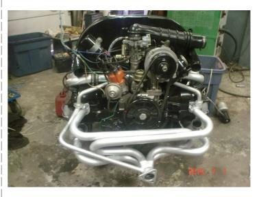
If you run a centre-mounted carb on a horizontally-opposed engine you need supplemental heat to insure proper vaporization in the runners. No mystery to any of this, it's in all the books and has been for seventy years.
