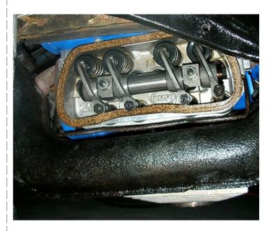
The less obvious reason has to do with the sealing surface around the valve gallery — the head surface against which the gasket is pressed to form the seal. If this surface becomes scratched or dinged — even slightly — it will not form an oil-tight seal. These scratches and dings usually occur when we adjust the valves.
