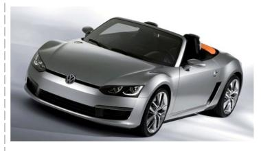
The 2009 Volkswagen BlueSport concept was just under four metres in length and powered by a 132 kW turbo diesel engine mounted in the rear, behind the two front seats. It was to be the first mid-engined VW since the VW-Porsche 914 of the early 1970s.
