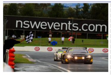
produces 425 kW. It has a six-speed sequential gearbox and is rear-wheel drive – NOT 4WD. The reason is that it was built for the European GT3 championship for production sports cars, and the GT3 rules outlaw AWD.
