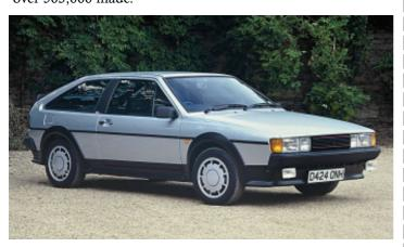
The Scirocco II (VW Type 53B) appeared in 1982, completely redesigned except for using the same A1 platform, and again built by Karmann. It was more powerful than the previous Scirocco, with the Euro-only 16V 1.8 engine producing 105 kW. Because VW Australia stopped selling
