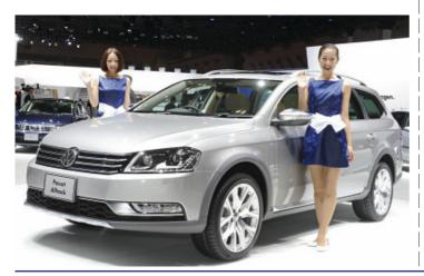
breakaway angle (significant when crossing the crest of a hill) from 9.5 to 12.8 degrees. Ruggedly styled front and rear bumpers increase the approach angle from 13.5 to 16 degrees, and the departure angle from 11.9 to 13.6 degrees.
