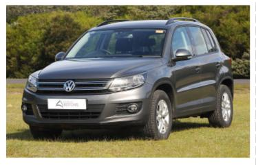
For the more adventurous that like to head off the bitumen occasionally, Tiguan will get you further than most of its peers, but it is still only a compact size SUV so serious rock crawling is out of the question. Volkswagen's electronically controlled 4Motion system is a sophisticated and well proven all-wheel-drive system. Regrettably, Tiguan only carries a space-saver spare wheel.
