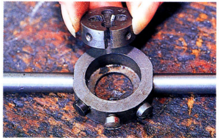
Stocks usually have three screws. Outer ones locate die in holder and centre allows small adjustment for the first cut.
