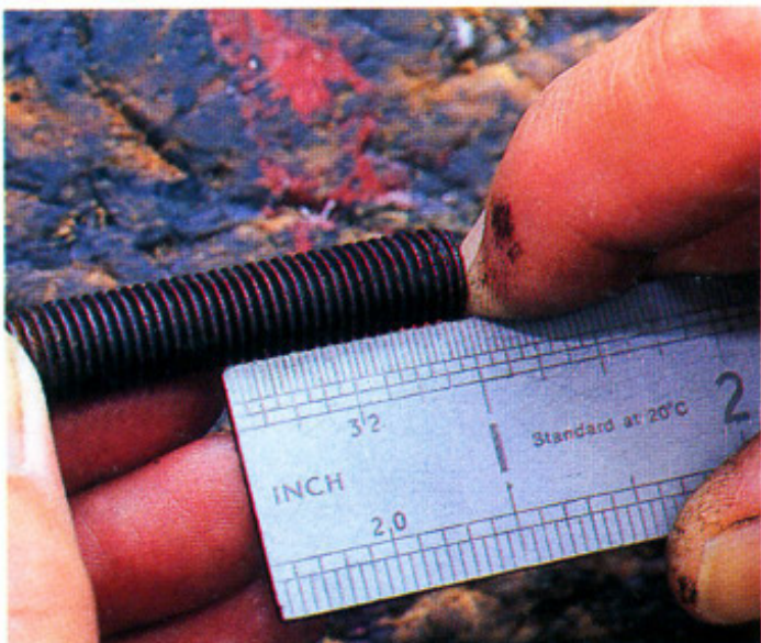
If you don't have a gauge and bolt diameter is imperial, use a ruler to count the number of threads per inch.
