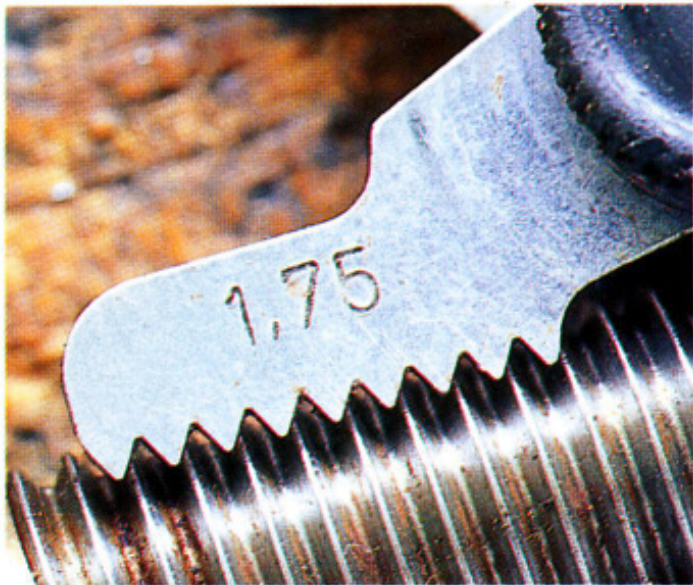
Metric pitches are measured in mm between thread peaks and are harder to establish without a gauge.
