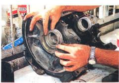
Collar on shell bearing takes up crankshaft thrust. Check there is no play between bearing and journal.
