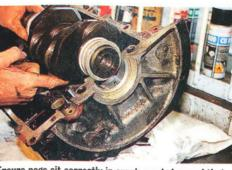
Ensure pegs sit correctly in crankcase holes, and that they locate in bearing shells when you lower the crank.
