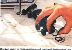
Rocker gear is over-engineered and well lubricated, so should last well. Check spring washers: they can snap.
