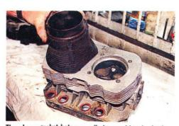
There's no gasket between cylinders and heads. Apply grinding paste and rotate cylinder under its own weight.
