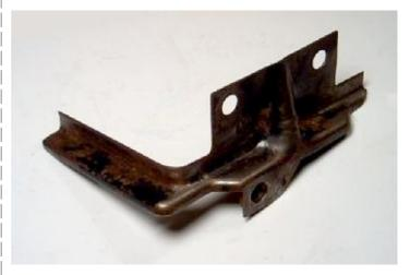
You don't have to remove the fastener to remove the fan shroud, just loosen it. The fastener is usually a slot head machine screw, as for the other tin-ware. (I like to use bolts instead of screws.) It should have the large diameter washer plus a warpy washer. It fits in the notch just beside where the air-vane return spring is fastened.
