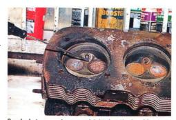
Cracks between valves are alright, but the head is scrap if cracked between the spark plug hole and exhaust valve.
