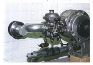
engine and causes less wear and tear on components. It also precludes the need to add oil to the air/fuel mixture to lubricate the vanes, as in the case with the Judson. A separate oil feed is take from the oil-pressure switch to lubricate the shaft of the Shorrock.
