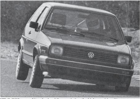
VW Golf lifts one of its wheels while negotiating the high-speed handling test.
