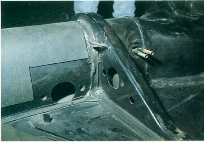
Genuine rhd chassis has pedal reinforcement plate with internal tapped threads.
