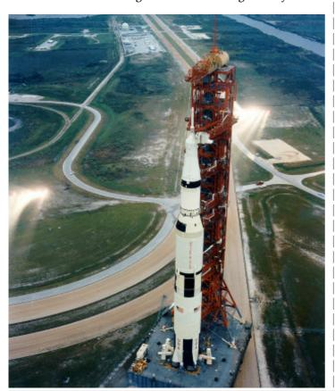
dead weight of empty fuel tanks any higher. Then the smaller second stage would fire and burn until it was empty, then it too was cast off. The much smaller third stage took the much reduced ship into orbit, and on the Apollo missions was then used to blast the ship away from orbit and onto the moon – the so-called Trans Lunar Injection burn. The first two stages fell back into the ocean or burned up in the atmosphere, and the third was discarded on the way to the moon.
