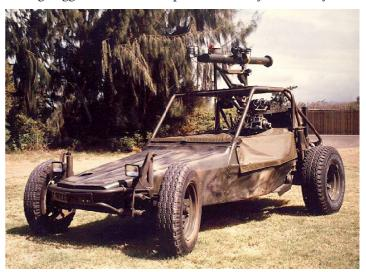
The DPVs had a payload capacity of 680 kg of military gear, and fully laden (2,250 kg) they could accelerate from 0 to 50 km/h in just four seconds, thanks to their powerful engines, light construction and low gearing. They had a top speed of 130 km/h, and with a standard off-road 80-litre fuel tank, had a range of around 380 km in desert conditions. An extra fuel bladder could extend the range to over 1,600 km.
