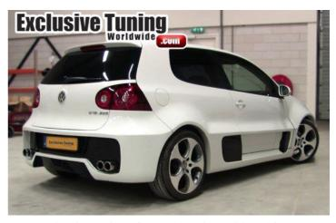
The kit consists of new side skirts, widened front and rear guards, a reworked hatch and bumper, along with an oddly proportioned front bumper and 'W12 650' badging, all used to create a close facsimile of the show car.
