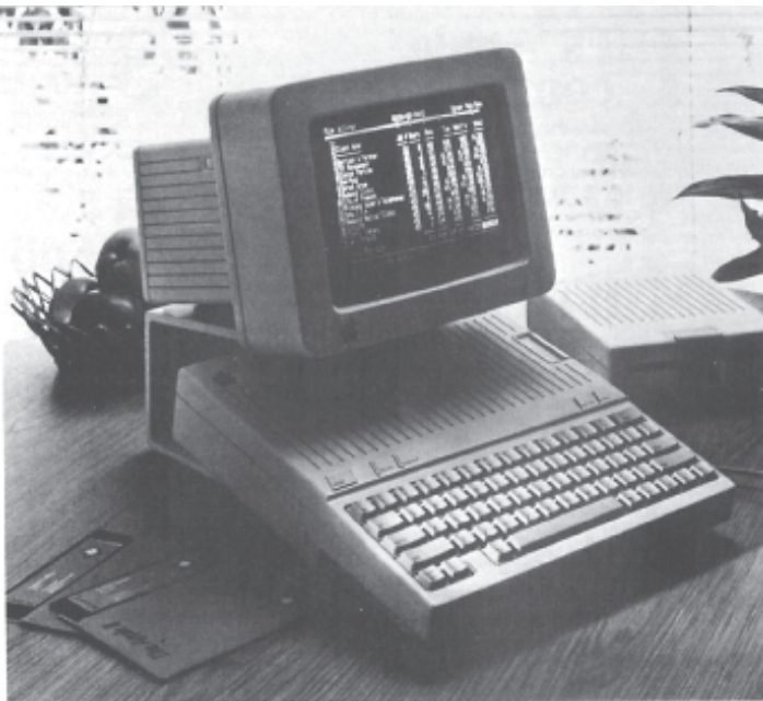
The Apple IIc personal computer, with mouse operation, built-in disk drive and IIc monitor. It runs most of the 30,000 estimated software programs for Apple II.
