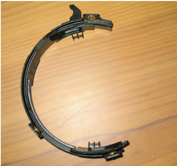
Above: Overall view of locking ring, showing the operating lever at the top.
