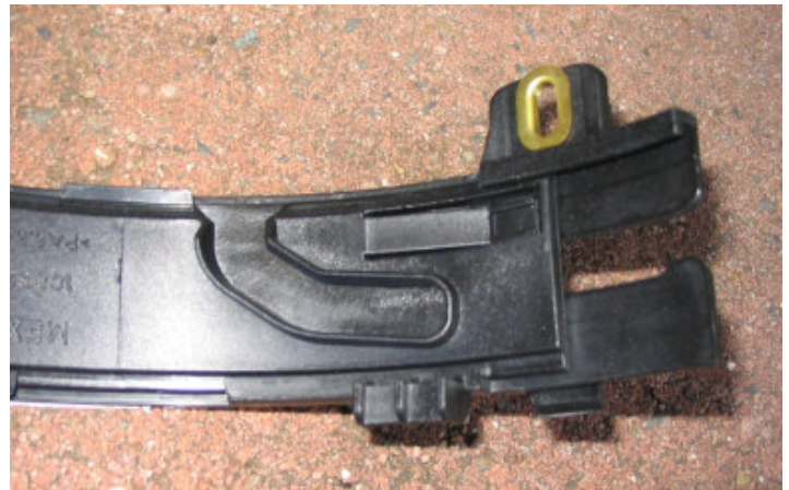
Above: Close up of the track that engages a lug on the headlight assembly. There are two of these. Lots of friction here.
