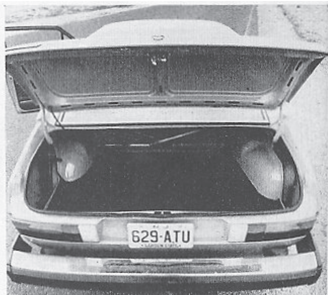
Wheel-housing intrusion is minimal in Dasher trunk, which offers more than 16 cubic feet of useful space, with a flat floor. Lifter is a reasonable 29.5 inches.
