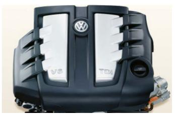
The new V6 TDI engine is 440 mm long, meaning that it is extremely compact. The cylinder crankcase features an angle of 90 degrees and is made from high-strength yet light vermicular or compacted graphite cast iron (CGI). This offers greater strength although it weighs 15 percent less than grey cast iron. The engine weighs only 220 kilograms; its cylinder gap is 90 mm and the compression ratio is 17.5:1.
