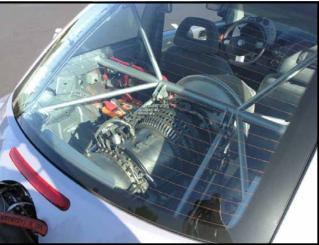
The first thing I did when I got the car was to cut the hole in the back for the engine. Made a fancy jig out of a tripod, a rod, and a lawnmower wheel to mark out the cut and went at it with a pneumatic saw. Then
