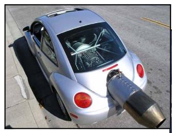
"Jet Under Glass". Air for the jet enters the car through the two side windows and the sunroof. It's a little windy inside but not unbearable.
