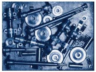
"All the screws used to be galvanized as white as these ones," he says, "But this type of screw isn't made anymore. Nowadays they're only chrome-plated yellow." So for the restoration work, each screw is sand-blasted individually and its surface is treated. Many other parts, large and small, receive the same treatment because the engines Dieter Wurster restores have to be original down to the last detail.
