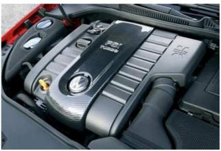
This 1984cc engine offers 147kW of power and 280Nm of torque with judges commenting on the excellent balance it displays between advanced technology, performance and economy - this is no wonder given the quality engineering work completed.
