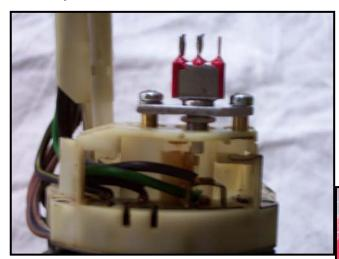
Above: the micro switch installed in its correct location.
