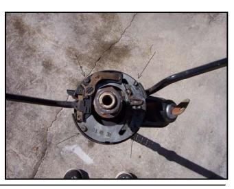
Previous page: A column I had that had been previously removed from a car. When the steering wheel is removed you'll be confronted with this picture. Note: the four screws that hold the assembly into the column.
