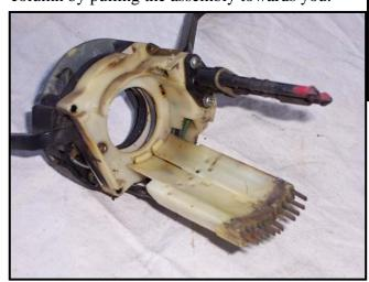
Above: is the indicator assembly as removed from the car, ready for modification.
