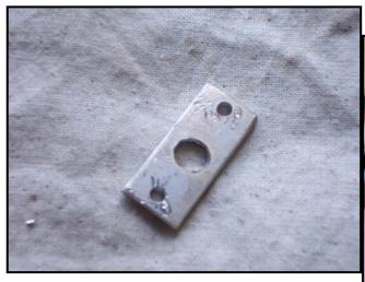
Above: My small aluminium plate drilled and cut to size. See further on in the article how one corner needs to be filed off to allow the switch assembly to fit inside the column assembly.
