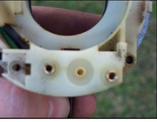
Above: Before the centre hole was drilled out to accommodate the switch.
