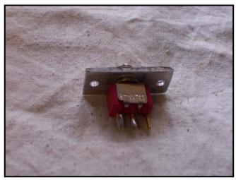
Above: Insert the micro switch into the middle hole of the aluminium and screw the switch up tightly.
