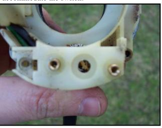
Above: After the hole has been enlarged to accommodate the switch.
