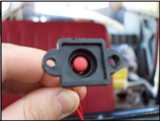
Above is the rear view of the switch. Note all terminals are numbered as per Volkswagens standard design. Also note the switch insert protruding from the back of the switch. This is the piece that needs to be carefully trimmed to size
