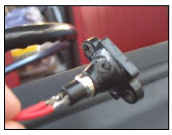
section from the rear of the switch and remove the plunger arrangement that is no longer needed.
