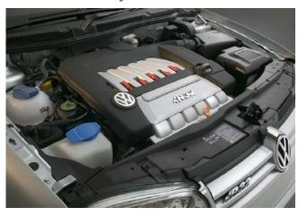
Golf R32's 24-valve V6 engine is distinguished by its very acute 15-degree V angle. The engine is a development of Volkswagen's 2.8-litre V6 with several changes to achieve significantly boosted power and torque.
